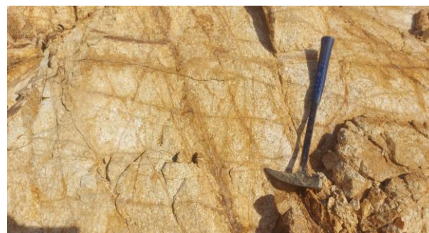
Figure 6. Stockwork-style sulfide veinlets formed within hydrothermally altered host rocks at the Demirli deposit
