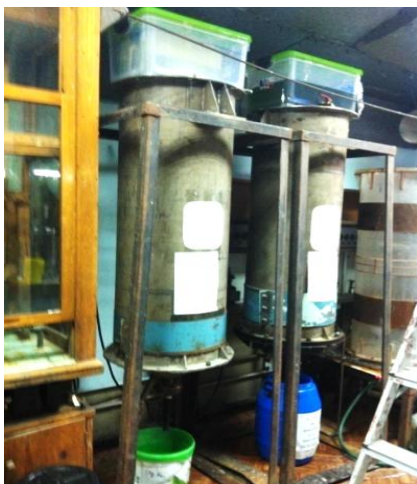
Figure 3. Laboratory setup for ore leaching tests conducted in titanium percolation columns
