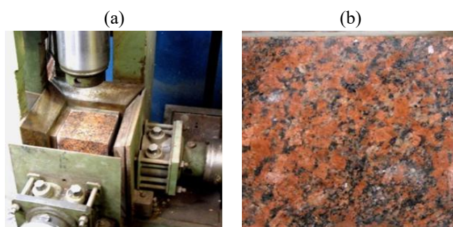
Figure 2. Exterior view of the working chamber (a) for loading samples and a granite sample (b)
