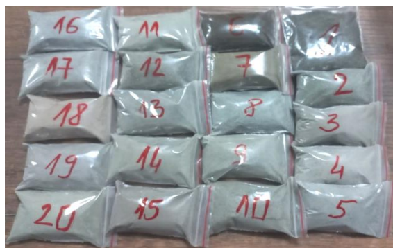
Figure 5. Prepared rock samples after grinding and sieving to a particle size of \leq 63 \mu\text{m} and weighing 10 g for laboratory analyses
