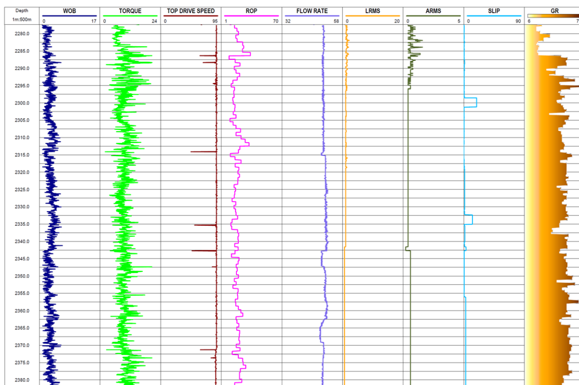
Figure 4. Depth profiles of downhole vibration metrics (LRMS, ARMS, Slip) and drilling parameters for well No. 2 over the 2280-2380 m interval (stable regime with alternative bit design)
