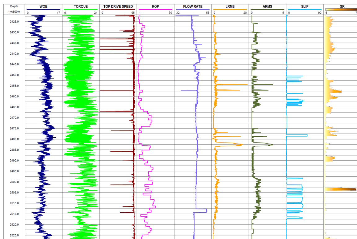
Figure 6. Depth profiles of downhole vibration metrics (LRMS, ARMS, Slip) and drilling parameters for well No. 2 over the 2425-2525 m interval (suppression of stick-slip vibrations by the alternative bit design)
