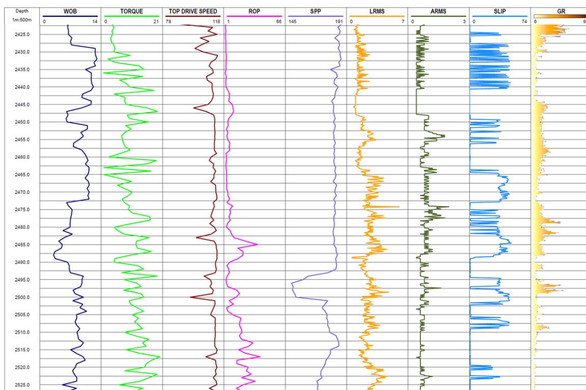
Figure 5. Depth profiles of downhole vibration metrics (LRMS, ARMS, Slip) and drilling parameters for well No. 1 over the 2425-2525 m interval (development of intense stick-slip vibrations)
