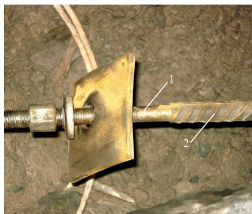
Figure 5. Rock bolt used: 1 – deformed steel bar; 2 – threaded section, where failures are typically observed
