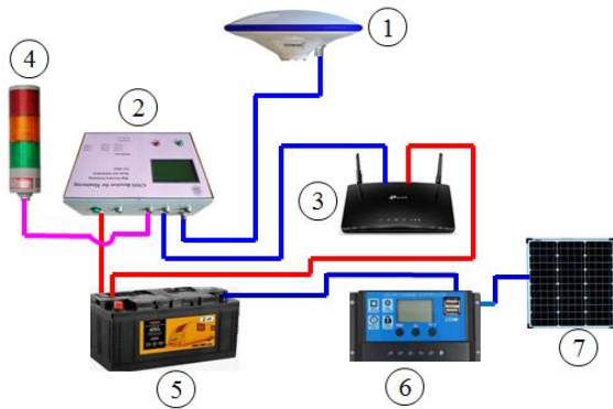
Figure 3. Components and their connection diagram in the real-time landslide and displacement monitoring station system: 1 – GNSS antenna; 2 – GNSS receiver; 3 – WiFi modem with 4G SIM card; 4 – alarm and signaling module; 5 – 12V battery; 6 – solar energy-charged controller; 7 – solar panel
