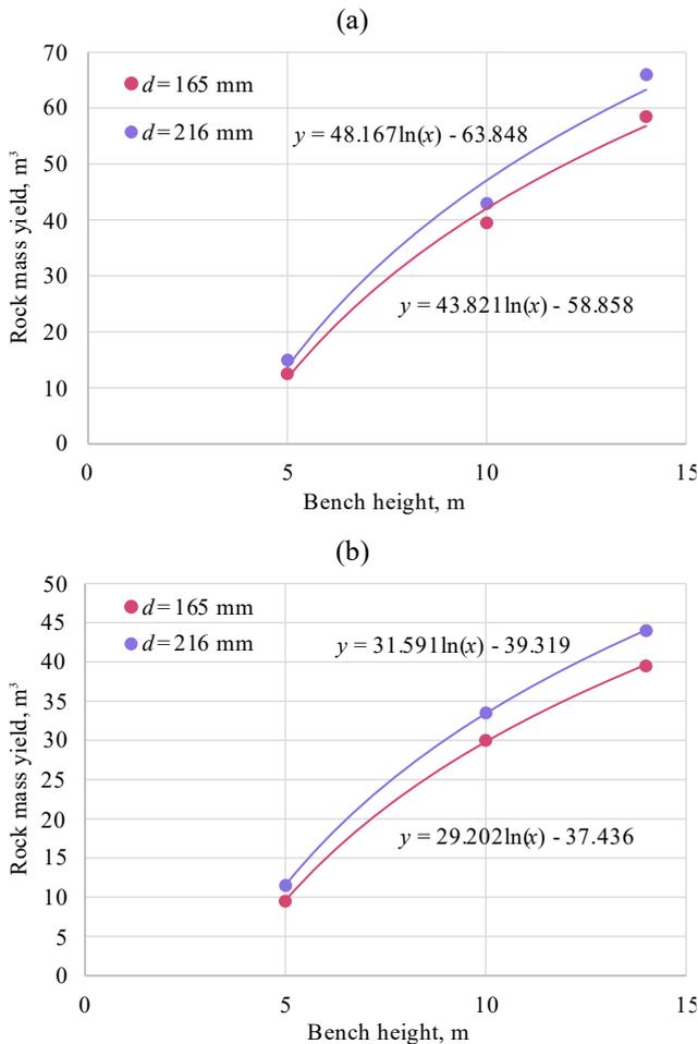
Figure 7. Dependence of rock mass yield from 1 linear meter of blasthole on bench height at different charge diameters: (a) for moderate-to-explode rocks; (b) for hard-to-explode rocks
