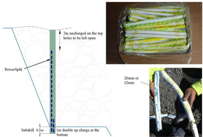
Figure 4. Example of a continuous split-forming product with a 10-m detonating cord
