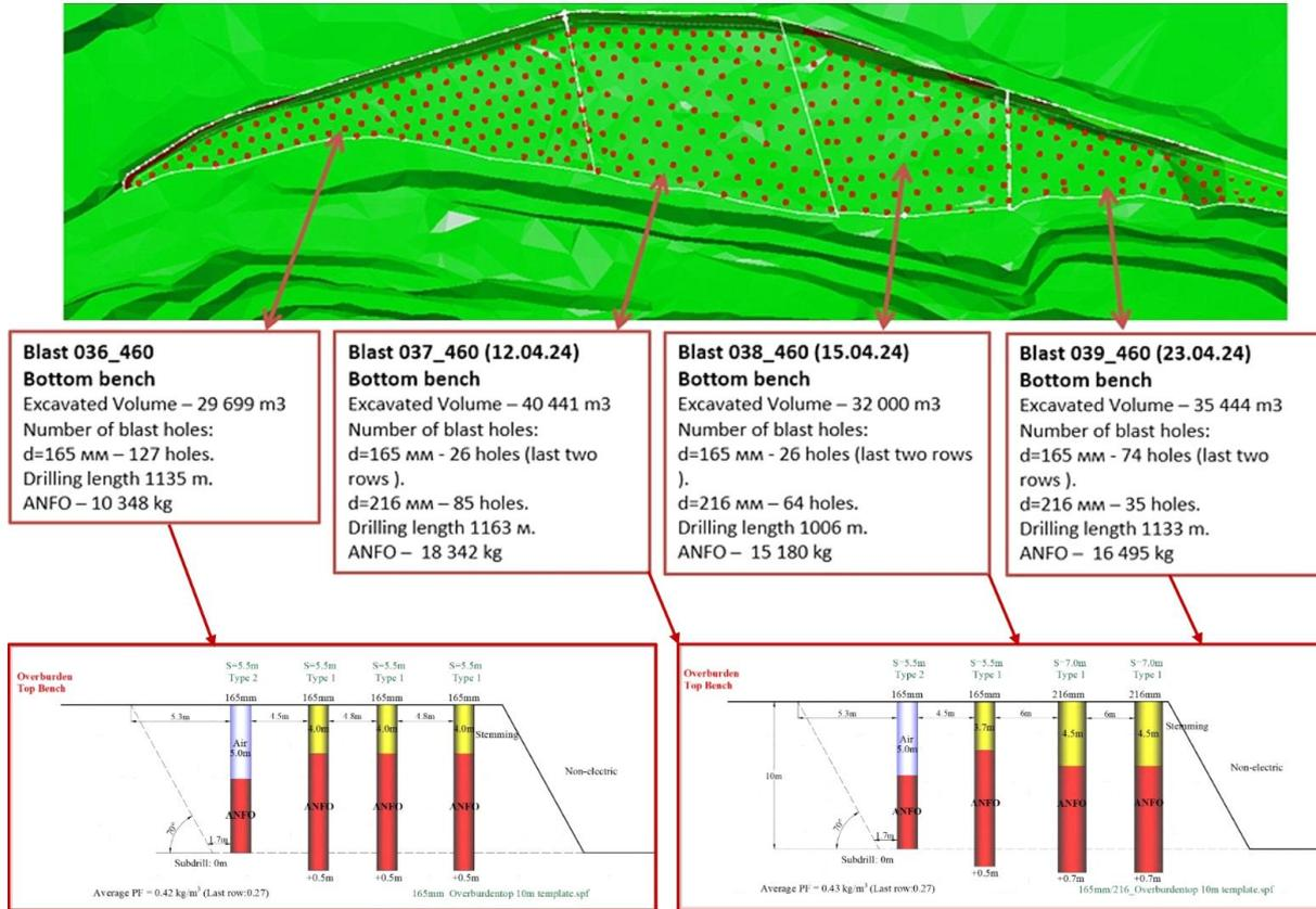
Figure 2. ayou of blasthole charges and parameters of test blasts on the block 460 upper benches of Pustynnoye field quarry
