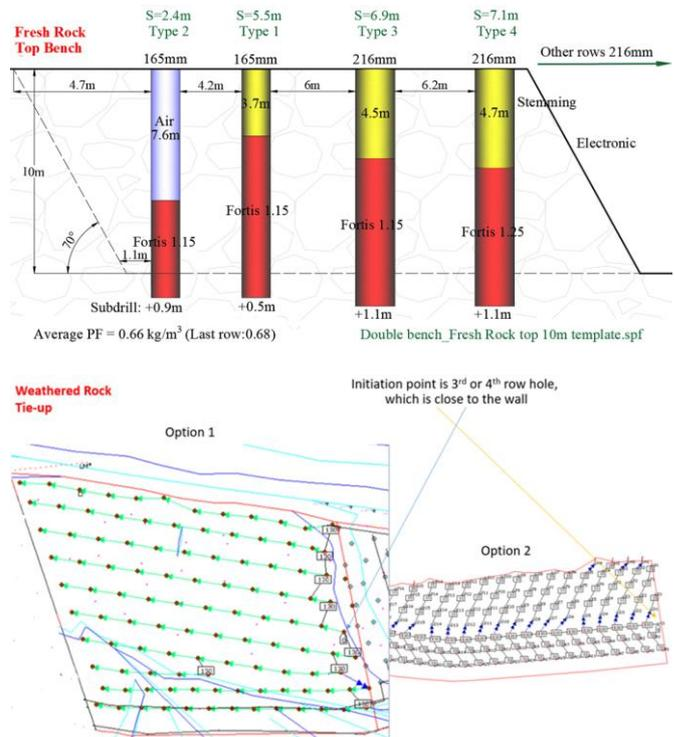
Figure 5. Near-wall blast projects using contour blasting: (a) blast-hole charging scheme for fresh rock; (b) options for schemes for linking blasts in the weathered rock zone
