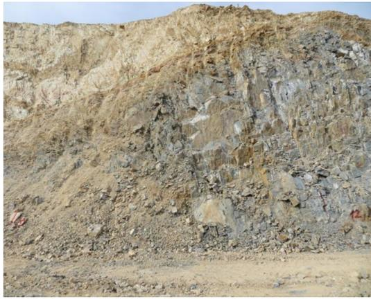
Figure 3. Mixing of primary rocks with surface rocks as a result of blasting
