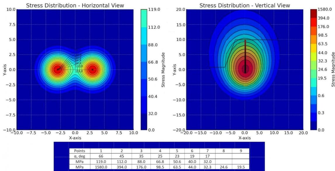
Figure 1. Stress distribution in the rock mass during blasting of blasthole charges on a bench
