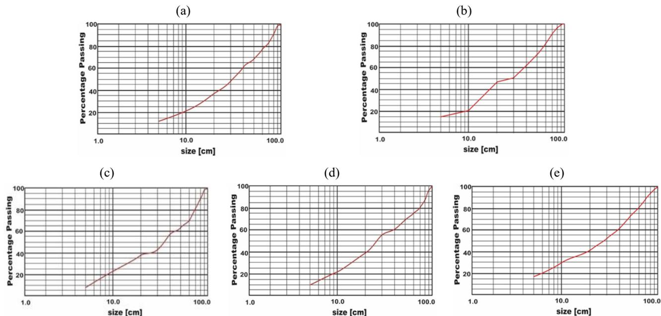
Figure 7. Cumulative grain size curves of image analysis of blasts A – E at OP2
