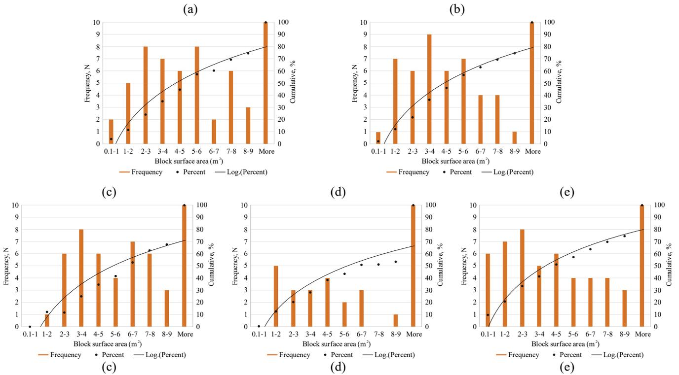
Figure 4. Cumulative graph of in-situ block size distribution for blasts A – E at OP1: (a) block A; (b) block B; (c) block C; (d) block D; (e) block E
