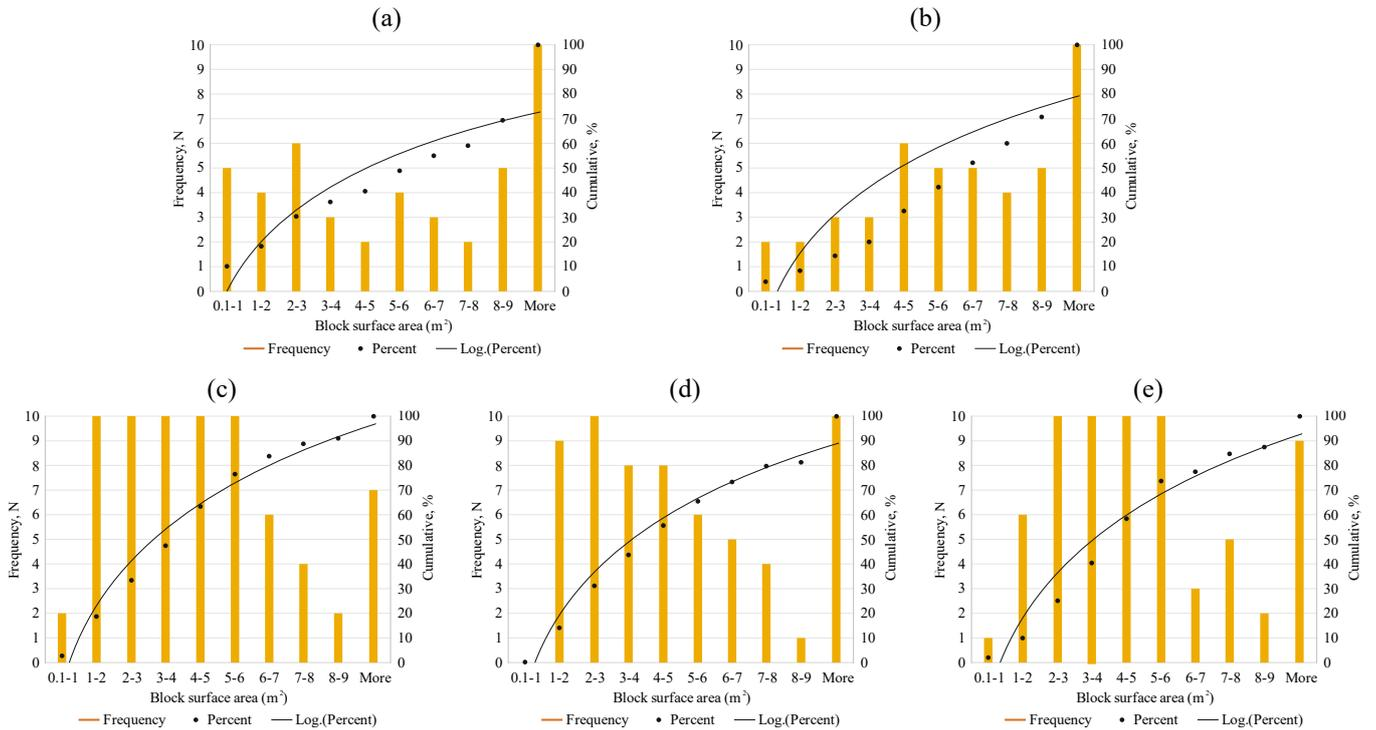
Figure 5. Cumulative graph of in-situ block size distribution for blasts A – E at OP2: (a) block A; (b) block B; (c) block C; (d) block D; (e) block E
