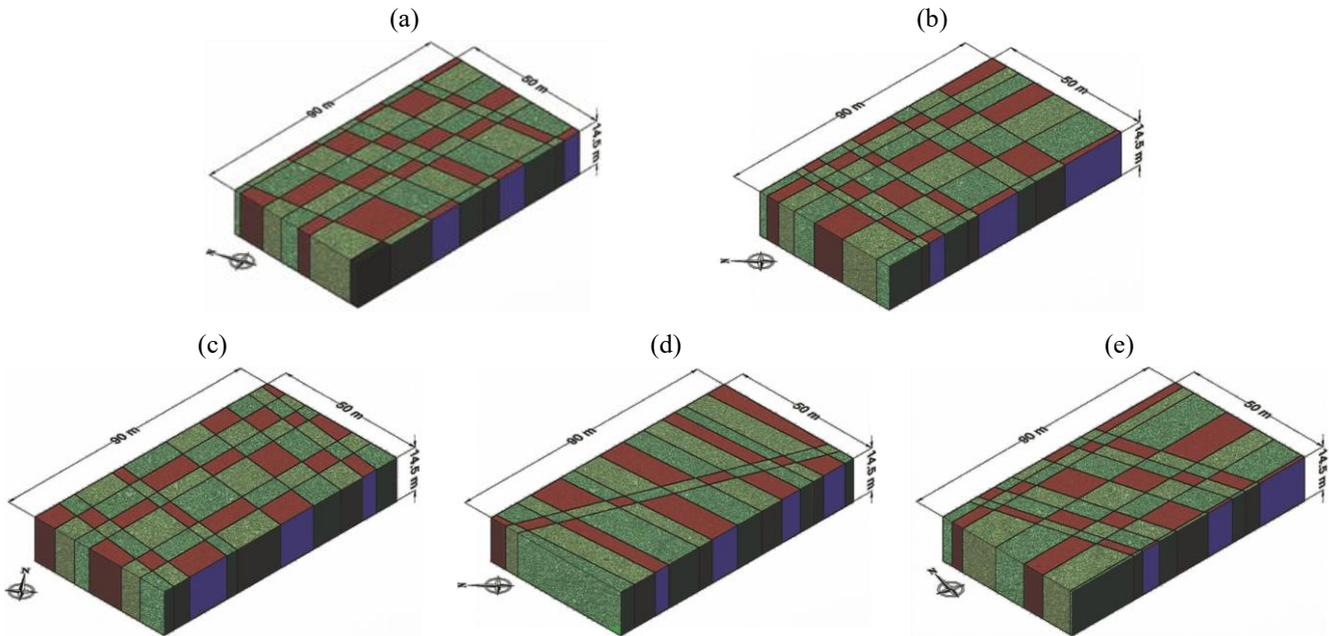
Figure 2. AutoCAD Block Size Distribution of Blasts A – E at OP1
