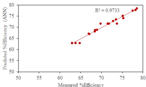
**Figure 8.** Comparison of the measured and predicted blasting efficiency using ANN
