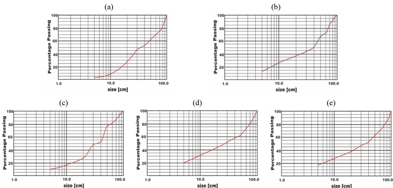
Figure 6. Cumulative grain size curves of image analysis of blasts A – E at OP1
