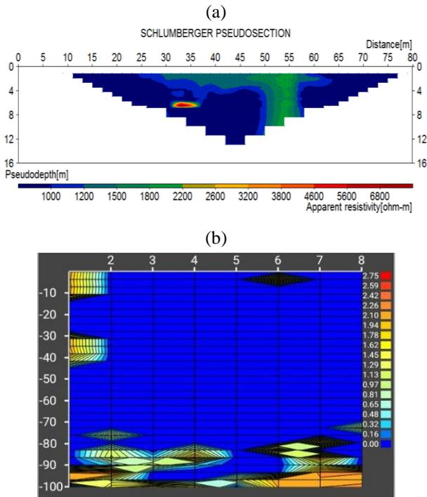
Figure 9. Structural analysis along the profile line P2: (a) Pseudosection showing apparent resistivity with anomaly picked at 50-55 m (Abem SAS 4000 series); (b) PQWT confirming the presence of structures seen in apparent resistivity from 50 to 58 m which is a possible conduit solute contaminant
