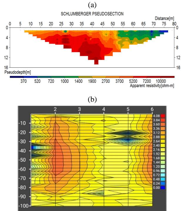
Figure 11. Structural analysis along the profile line P4: (a) Pseudosection showing apparent resistivity with high anomalous bodies (Abem SAS 4000 series); (b) PQWT profile line confirming the structures seen from ABEM profile line around point 35 to 42 m sandstone exposure to the near-surface to 100 m deeply seated
