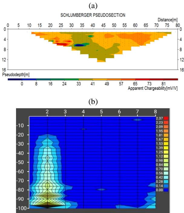
Figure 10. Structural analysis along the profile line P3: (a) Pseudosection showing apparent resistivity with some sparse anomalous bodies (Abem SAS 4000 series); (b) PQWT profile line showing the structure to be extensive vertically at point 25 to 33 m
