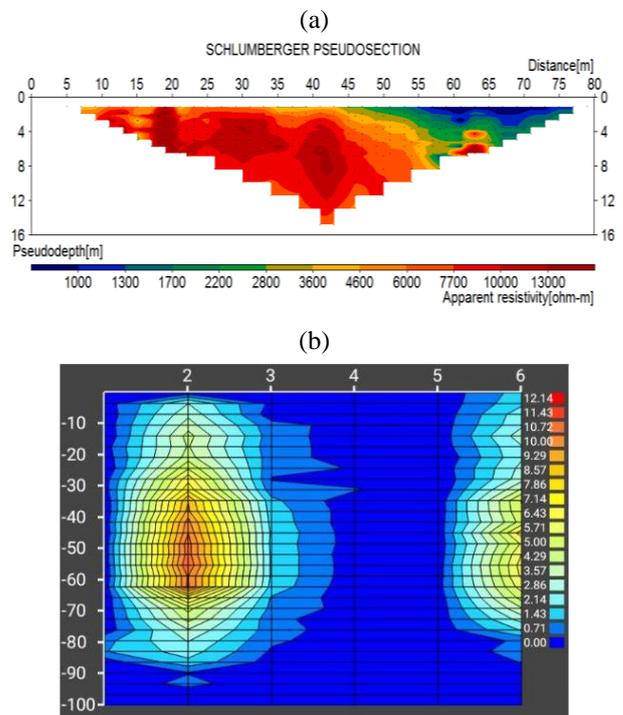
Figure 12. Structural analysis along the profile line P5: (a) Pseudosection showing apparent resistivity of anomalous bodies (Abem SAS 4000 series); (b) PQWT profile line confirming the structures seen from ABEM profile line around point 40 to 46 m, which could serve as a conduit for water seepage in a sandstone environment
