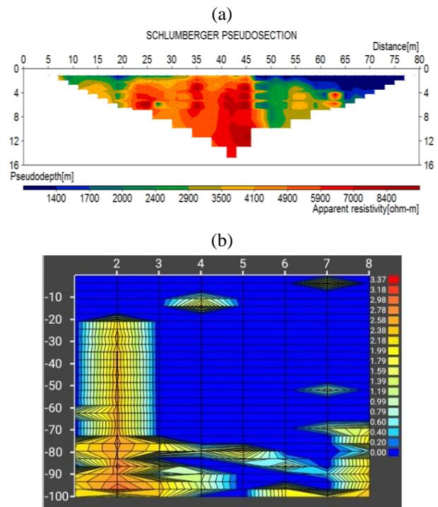
Figure 8. Structural analysis along the profile line P1: (a) Pseudo section showing apparent resistivity with some anomalous bodies 20-45 m horizontally running (Abem SAS 4000 series); (b) PQWT profile line confirming structures seen while running ABEM profile around point 42 to 50 m which could serve as a conduit for water seepage in a sandstone environment
