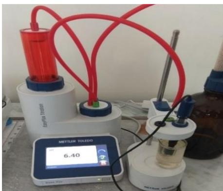
Figure 5. Photofixation of research process for determining acidity in leaching solutions without the use of surfactants
