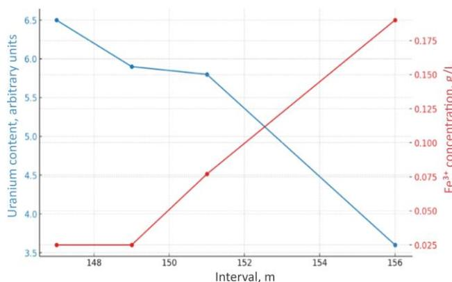
Figure 6. Results of core material testing (uranium and Fe<sup>3+</sup> concentration) for horizon intervals
