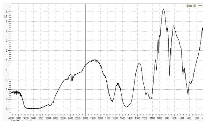
Figure 2. IR spectrum of leaching solution using OP-10
