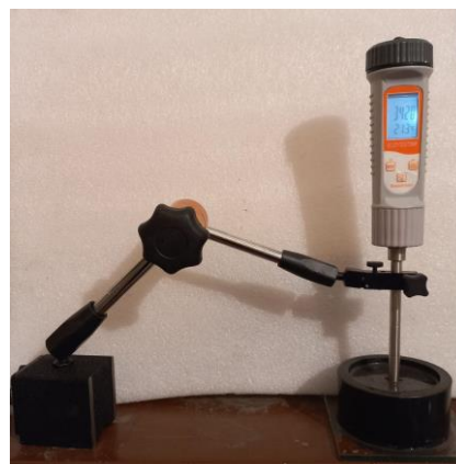
Figure 8. Monitoring of electrical conductivity values of the paste backfill mixture using a BT-761 conductivity meter
