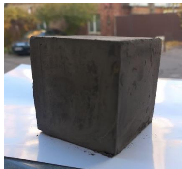
Figure 5. Hardening of cubic paste backfill mixture samples in the ambient environment
