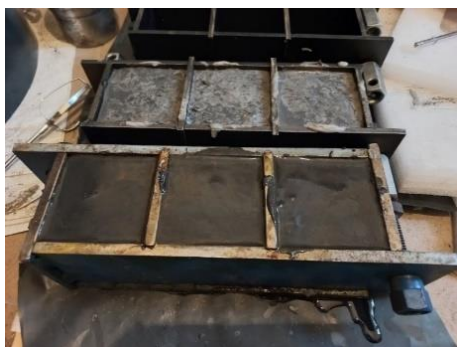
Figure 4. Paste backfill mixtures placed in metal molds 3FC-70
