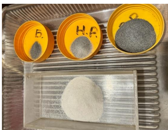
Figure 4. Photo-fixation of samples from Syniavske granite deposit after magnetic separation
