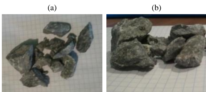
Figure 10. Rock samples taken from the unstable formations of Akbakay deposit: (a) are small rock fractions (i.e. 5-10 mm); (b) are large rock fractions (i.e. 15-20 mm)
