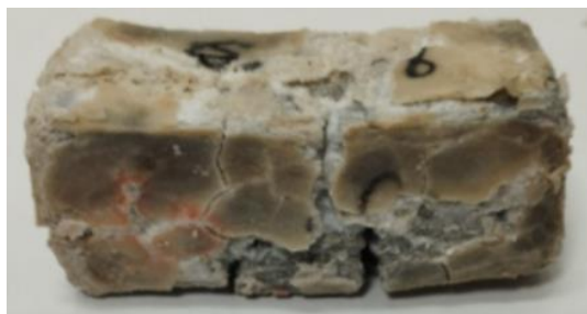
Figure 6. A sample of cement stone under the influence of sulfate-magnesium corrosion
