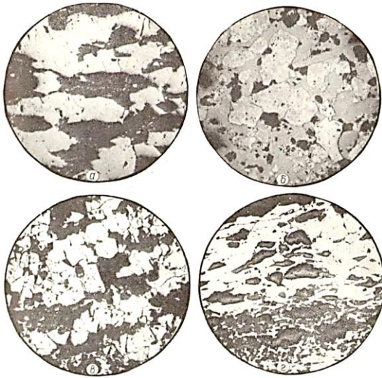
Figure 1. Structural peculiarities of iron-containing minerals: (a) lancetonide hematite; (b) martite with relics of magnetite; (c) euhedral-grained magnetite segregations in the hornfels; (d) the relationship of hematite (white) and magnetite (gray)
