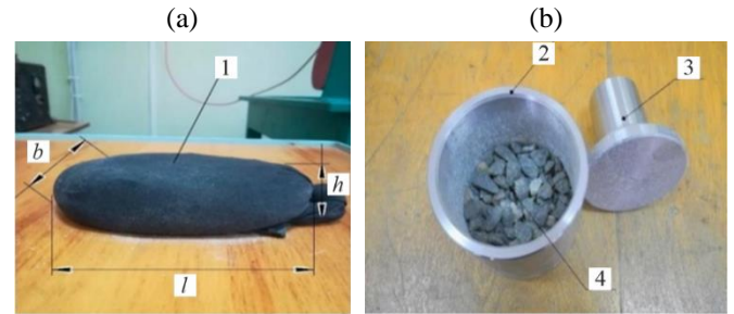
Figure 2. Experimental models for studying deformation properties of broken rock under static load conditions: (a) for uniaxial compression with lateral expansion; (b) for compressive stress of the source material; 1 – fabric shell on the broken rock; 2 – steel cylinder; 3 – plunger; 4 – broken rock; b – sample width, m; l – sample length, m; h – sample height, m
