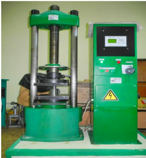
Figure 1. General view of hydraulic press П-50 for determining deformation characteristics of the backfill material made of broken rock
