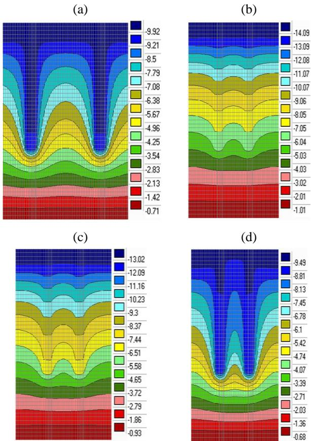
Figure 3. Isolines and isofields of vertical displacements (s), mm: (a) reinforced auger micropile (variant 3); (b) soil-cement micropile (variant 1); (c) micropile made of the reinforced soil cement (variant 2); (d) reinforced auger micropile (variant 2)
