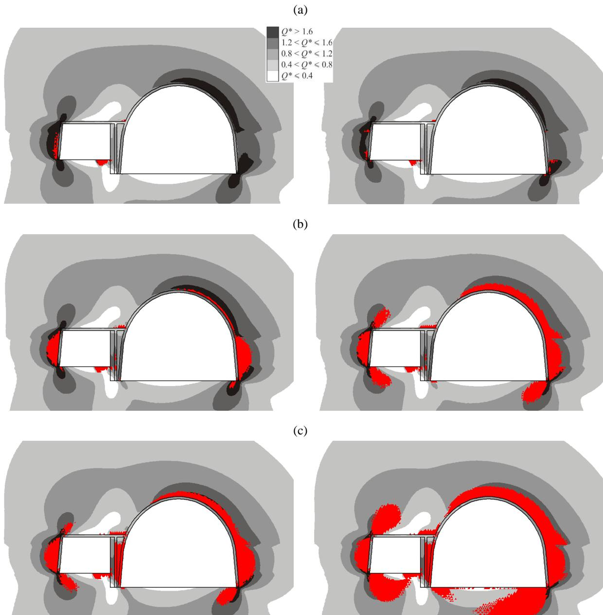
Figure 2. Zones of inelastic deformations, distributions of the  $Q^*$  parameter values within the rocks with average strength  $R_c = 33.5$  MPa (left) and  $R_c = 20.6$  MPa (right) around the refuge chamber with the basic support: (a)  $H = 400$  m; (b)  $H = 800$  m; (c)  $H = 1200$  m
