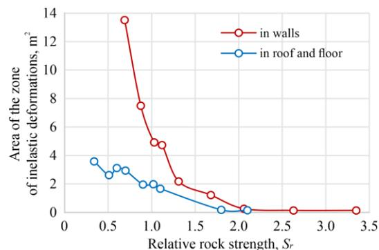
Figure 3. Area of the zones of inelastic deformation
