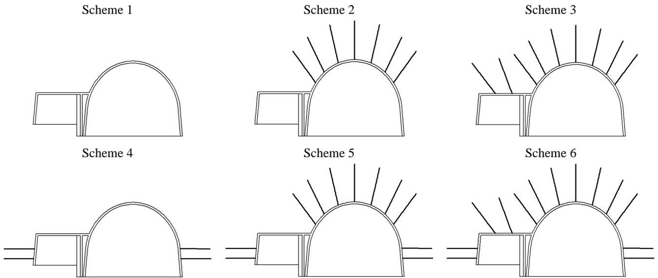
Figure 4. Schemes of the refuge chamber support
