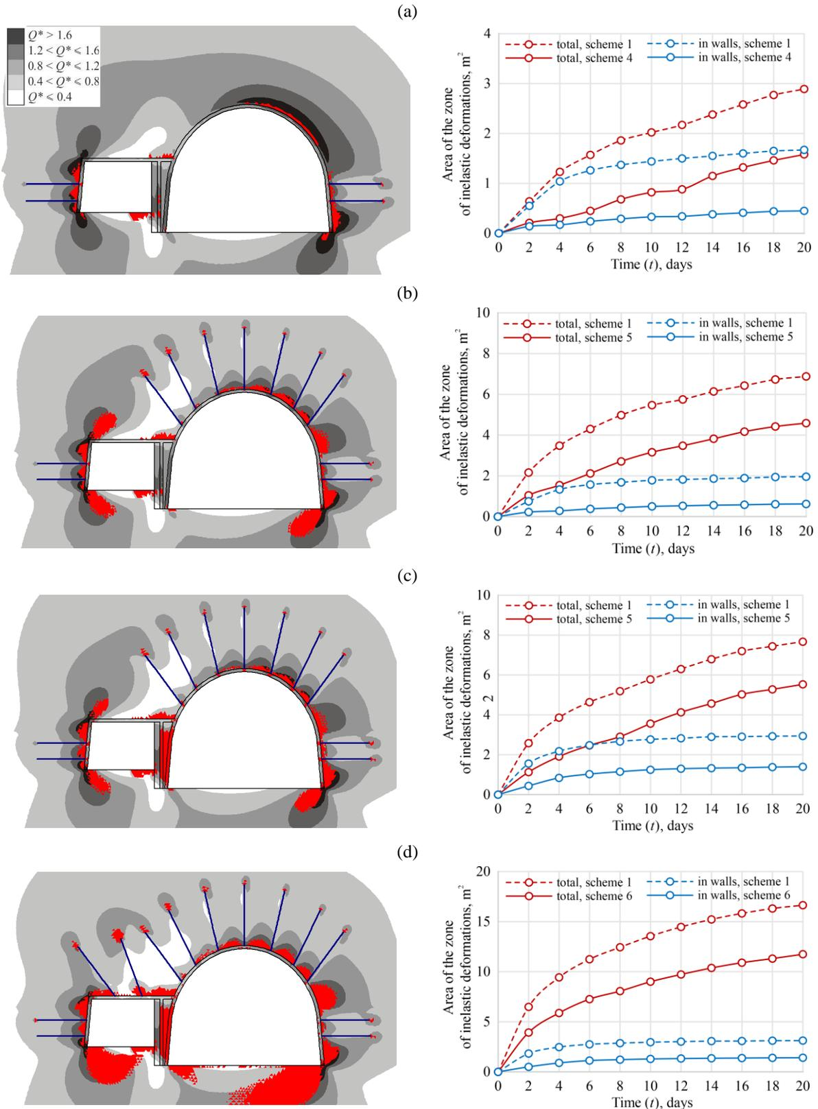
Figure 5. Zones of inelastic deformations, distributions of the values of  $Q^*$  parameter and graphs of changes within the area of the zone of inelastic deformations: (a)  $H = 800$  m,  $R_c = 33.5$  MPa,  $R_{c\ wall} = 21.14$  MPa; (b)  $H = 800$  m,  $R_c = 20.6$  MPa,  $R_{c\ wall} = 18.08$  MPa; (c)  $H = 1200$  m,  $R_c = 33.5$  MPa,  $R_{c\ wall} = 21.14$  MPa; (d)  $H = 1200$  m,  $R_c = 20.6$  MPa,  $R_{c\ wall} = 18.08$  MPa
